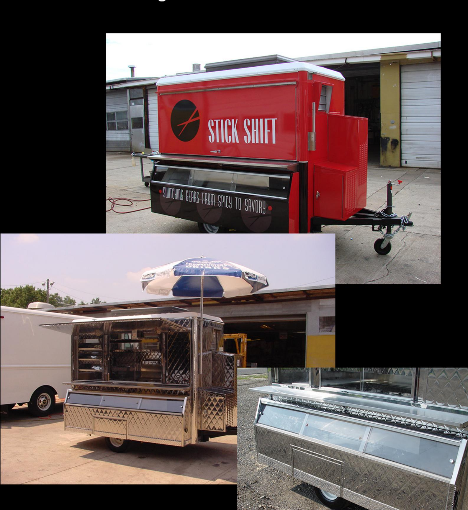
650 over-all dimensions: 96\text{\text{\text{VL}}} x 48\text{\text{\text{WV}}} x 96\text{\text{\text{H}}} (Dimensions do not include hitch or ice well extension) All tubular steel framing and under-carriage coated with a military grade rust inhibitor Completely enclosed Fiberglass roof Sliding plexi-glass service windows Stainless steel exterior Two pneumatic trailer wheels on automotive type springs
